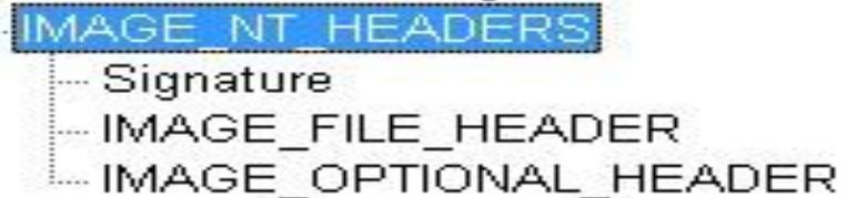
The diagram shows a tree view of the `IMAGE_NT_HEADERS` structure. The root node is `IMAGE_NT_HEADERS`, which is expanded to show three sub-nodes: `Signature`, `IMAGE_FILE_HEADER`, and `IMAGE_OPTIONAL_HEADER`.
